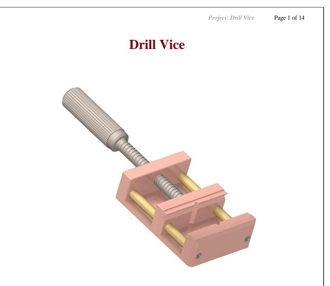
Make precise items by the measurements given on particular 2D drawings. The measurements are given in millimeters, and the measurements in inches are given in brakes (1 inch = 25, 4 mm).
